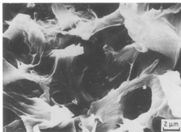
Figure 5 Fracture surface of quenched sample in the region of slow crack growth.
